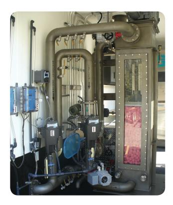
The pilot filter cell is 18" square and has a media depth of 30" without compression. The vessel and internals are constructed of 304 stainless steel. The area of the filter media face is 2.25 ft² and the flow at 30 gpm / ft² is 68 gpm. In some situations the flow may be as high as 40 gpm / ft² or influent flow of 90 gpm.
