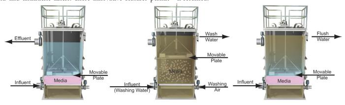
Filtration Cycle Wash Cycle Flush Cycle
